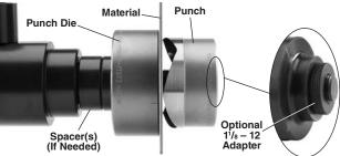
Figure 3 - Setting Up The Punch Head
