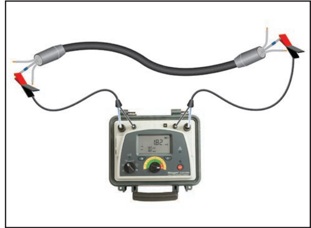
Fig 9: Conventional test, one kelvin at either end of a core of a multi-core cable
