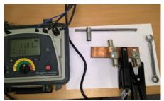
where electrical current is involved. Overtightening can cause the connection to become skewed, with less surface contact and higher resistance.
