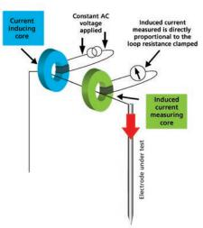
measurements. For the clamp-on method to work there must be a seriesparallel resistance path (and the lower the better). The more electrodes or ground paths in the system the nearer the measurement gets to the actual electrode under test's true resistance. The following figure shows a pole ground configuration, one of the most effective applications of the clampon ground tester.
