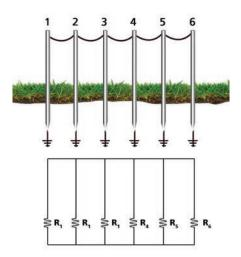
The circuit diagram for this configuration follows (based on a clamp-on ground tester being clamped around pole 6):
