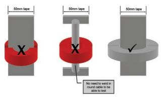
Some ground electrodes are secured quite close to the building wall or utility pole, making it difficult to clamp the head around the rod. The thicker the head, the more difficult this process is. A thinner head is preferable, if performance is not compromised.
