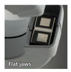
As mentioned in the section on potential sources of error on the previous page, dirt trapped between the closing gap in the clamp head can result in erroneous readings. Clamp-on ground testers are used outdoors in environments that are often dusty and dirty. They are exposed to materials that can end up on the core ends of the jaws. With flat core ends, the surfaces can be cleaned easily. This same material tends to get stuck in the interlocking teeth and is very hard to remove.
