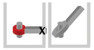
A larger inner area allows for clamping around larger ground rods or ground tapes (some of which can have a width of 50 mm). With a smaller internal opening on the instrument, the larger ground tape must be cut and a thinner copper bar welded in between to allow the instrument to make a measurement.
