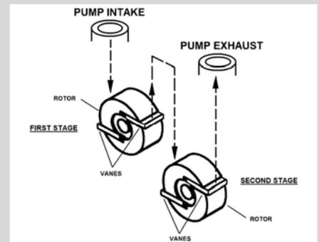
First stage exhausts into the intake of the second stage similar to two single stage pumps connected together.
