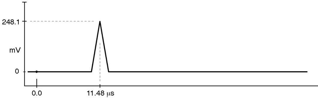
Figure 23: 525 Line Mod Pulse and Bar, R-Y
