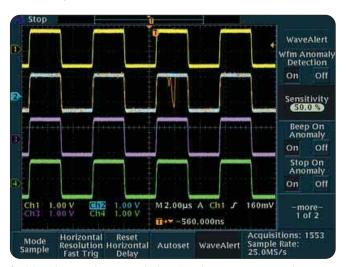
WaveAlert waveform anomaly detection alerts you to any waveform that deviates from the "normal" input such as the glitch on channel 2.
