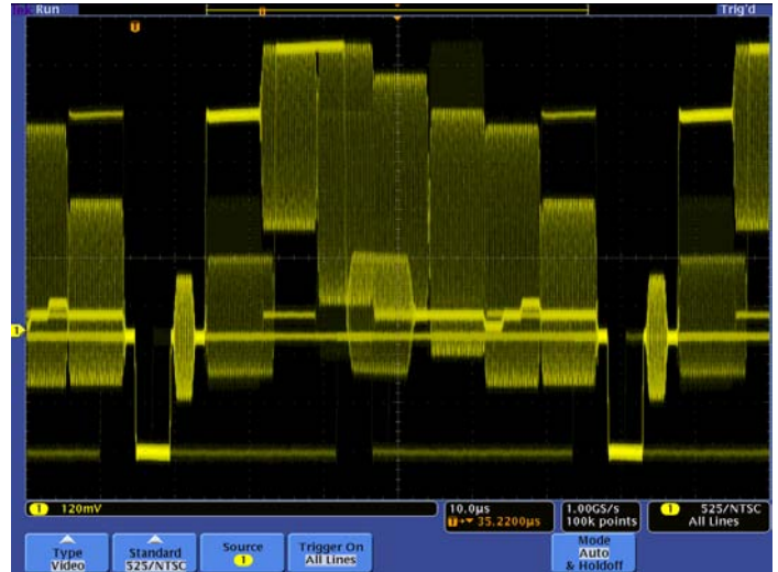
Viewing an NTSC video signal. Notice the intensity-graded view provided by the DPO's ability to represent time, amplitude, and distribution of amplitude over time.
