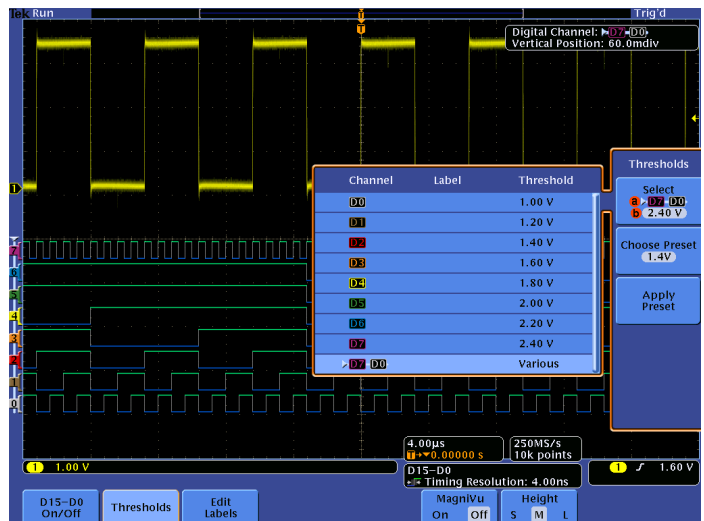
With the color-coded digital waveform display, groups are created by simply placing digital channels together on the screen, allowing the digital channels to be moved as a group. You can set threshold values for each channel, enabling support for up to 16 different logic families.
