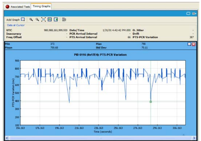
Advanced Timing Analysis including PTS-PCR for real-time buffer measurements to give indication of encoding and multiplexing errors.
