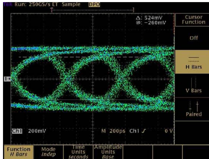
Figure 3-1: Typical eye-pattern of 20 m of Belden 1694A cable
