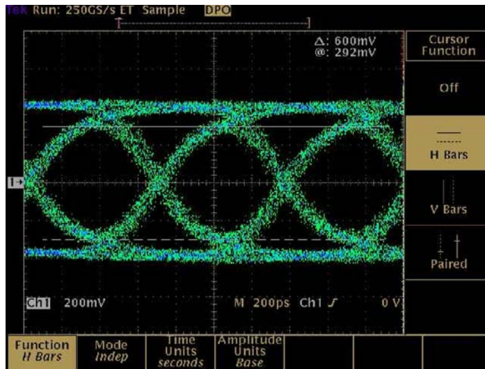
Figure 3-2: Typical eye-pattern of Channels 1-6 HD output (Channels 1-3 with Opt. ELSW)
