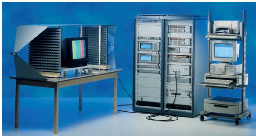
Typical application of RF millivoltmeters: field-strength measurement for the determination of EMS (Photo 43206-4)
