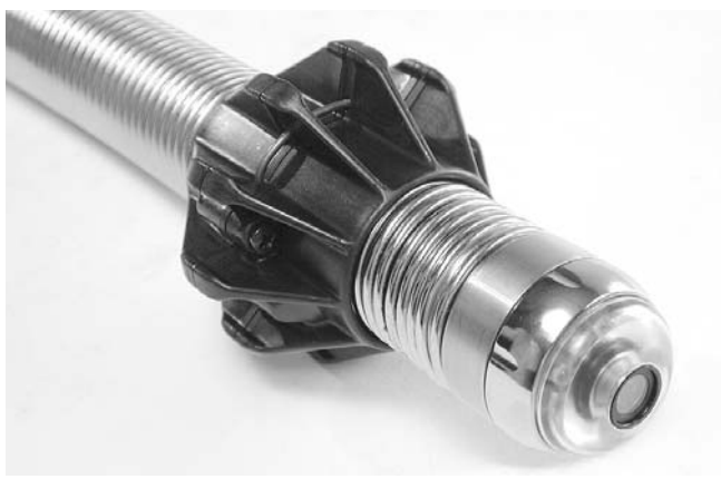
Figure 27 – Slide Ball Guide over spring and push Retaining Rings down to lock the guides in place.
