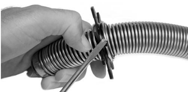
Figure 23 – Place flat tip of screwdriver between c-ring and base of spike and pry c-ring out of groove.
