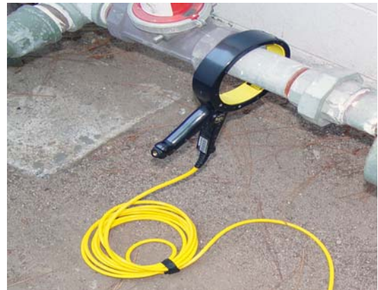
Figure 4: Example: Attaching the Inductive Clamp
