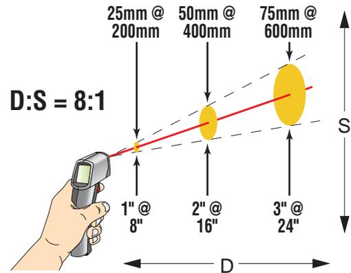
The MiniTemp thermometer is intended for close range targets, measuring a minimum target area of 1 inch in diameter out to a distance of approximately 8 inches, and has a 6 inch target measurement area at 4 feet.
