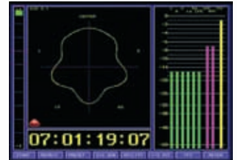
StarFish™ with phase correlation display, timecode and full 5.1, stereo & mono peak metering.
