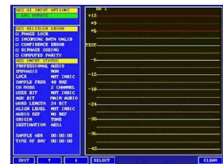
The bit status display supplies information about the content and the physical layer of the AES3 data signal.
