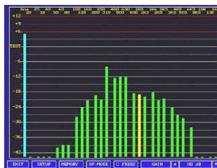
The 1/3-Octave spectrum shows the energy distribution of the input signal
