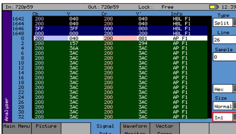
The Signal Data menu shows the video signal as a data stream in several formats as described below. In each mode, the data may be displayed in hexadecimal, decimal or binary formats. The binary format is not available in grid mode. The data may also be displayed as 10-bit or 8-bit format.
