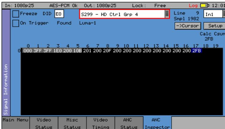
The SDI Data Option allows Ancillary data packets to be detected and checked for errors.
