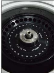
Rotor with built-in nut
