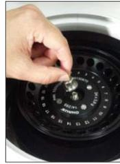
Rotor with separate nut
