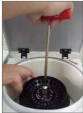
Tool for rotor with nut
