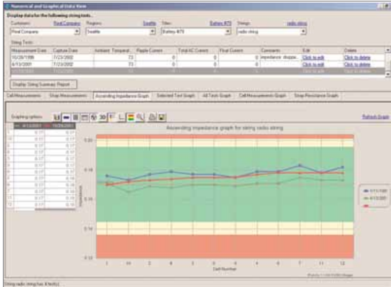
Figure 4: ProActiv ascending impedance graph with Pass/Warning/Fail bands
