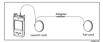
Figure 3. Connections for Launch + Tail Compensation
