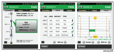
Figure 5. Examples of OTDR Results Screens
