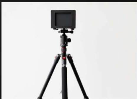
Photo shows tripod mounting of blackbody calibrator.
