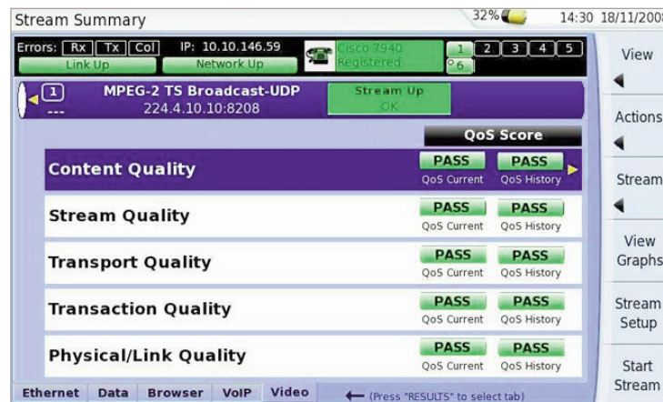
Figure 2: Example of Video test results using the T-BERD/MTS-4000 GUI with the JDSU Quality Layer Model
