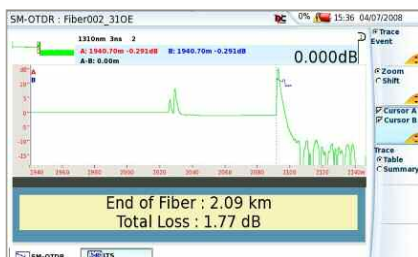
OTDR/fault locator screen
