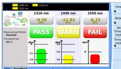
PON power meter screen
