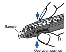
• Apply an appropriate amount of force at the position shown in the figure to squeeze th pincher arms around the sample. The contact resistance value will vary with the amount of force applied. The effect of contact resistance is particularly pronounced when measuring low-impedance elements or performing short correction.
