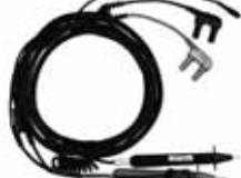
9465 PIN TYPE LEADS and 9466 REMOTE CONTROL SWITCH (Cable length: connector to fork 1.7 m, fork to probes 10 cm; coiled expanding section maximum 55 cm)
