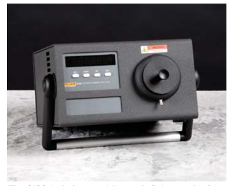
The 9133 includes a quick-attach fitting on the front bezel for dry air purging, which eliminates ice.
