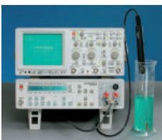
Precise temperature measurement with sensor HZ887
