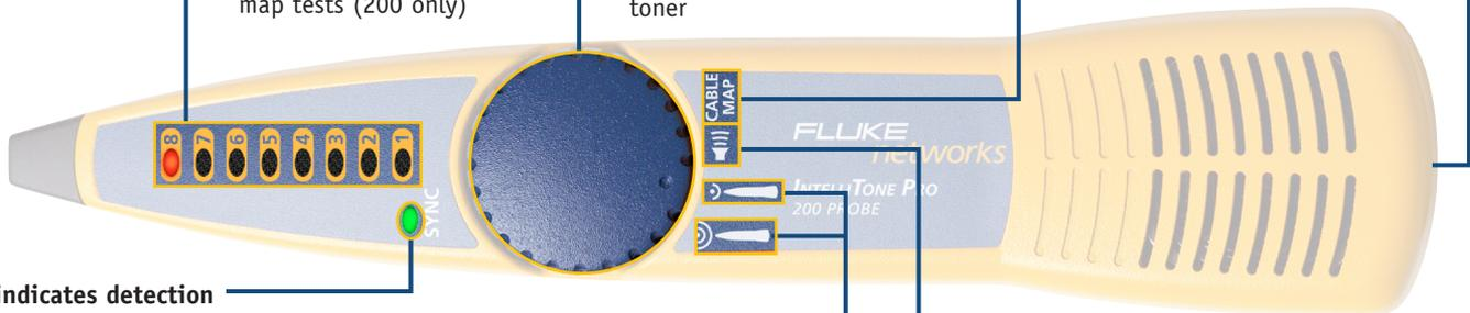
**SYNC indicates detection of IntelliTone signal** and shows battery status at power-up
