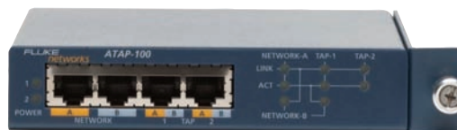
ATAP-100 Single port dual output Copper Aggregating Tap 100Mbps
