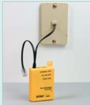
Transmitter injects traceable signal into cables, checks telephone lines, and performs continuity checks
