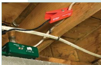
External NCV probe can be used to identify wiring in hard-to-reach areas where the transmitting unit cannot fit
