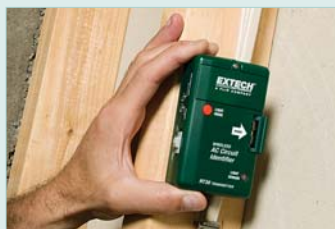
Clamp-on unit will sense AC Voltage of a mid-run wire and transmit the voltage present signal to the receiver indicator unit.
