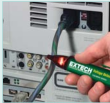
Locate power cord breaks
