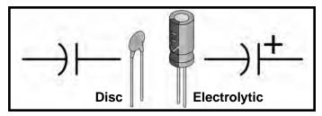
The *capacitance* (electricity storage capacity) of a capacitor is expressed in a unit called a *farad*. The farad is an extremely large amount of electricity, so the value for most capacitors is given in millionths-of-a-farad (microfarads).
