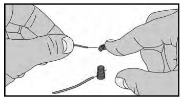
Sometimes you need to connect two or three wires to a single spring terminal, so be sure the first wire doesn't come loose when you add the second and third wires. The easiest way to do this is to push the spring on the side opposite side where you connected the first wire.
