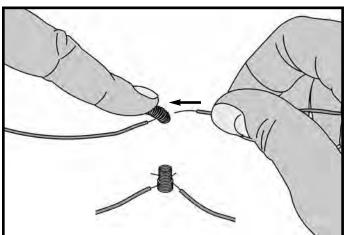
Be sure that you only insert the exposed, shiny part of the wire into the spring terminal. If the plastic insulation part of the wire is inserted into the terminal, electrical contact is not made. To remove the wire from the spring terminals, simply bend each terminal and pull the wires from it.
