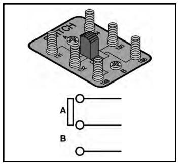
**Key:** The Key is a very simple switch - press it and the circuit allows electricity to flow through it. Release it and there is a break in the circuit's path, so the circuit is not complete. You will use the key in many circuits, most often in the signaling circuits (to send Morse code, and so on).
