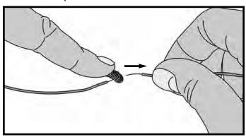
After a lot of use, the exposed metal ends of some of the wires might break off. If this happens, remove 3/8" of insulation from the broken end and twist the strands together. You can remove the insulation with a wire-stripper tool or a penknife. Be very careful doing this, as a penknife is very sharp.
