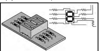
Integrated Circuit: As you might already know, after the transistor was invented in the middle 1940's, the next big breakthrough in electronics was the integrated circuit in the early 1960's. The great advantage of ICs (as we call them) is that the equivalent of hundreds or even thousands of transistors, diodes, and resistors can be put into a small package.
