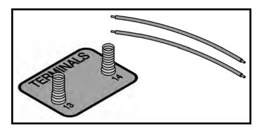
**Wires:** You will use the wires to make connections between terminals.
