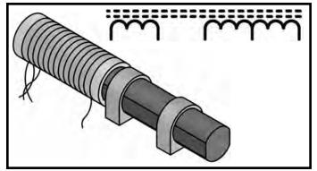
**Transformer:** If you wrap two wires from different circuits around different ends of an iron bar then a current flowing through the wire from the first circuit will magnetically create a current in the wire from the second circuit! If the second coil has twice as many turns (more magnetic linkage) as the first coil then the second coil will have twice the voltage but half the current as the first coil. A device like this is called a *transformer*.
