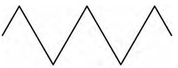
The shape of this wave comes from the slow charging of the  $0.1\mu F$  capacitor through the control and the  $100k\Omega$  resistor, and the capacitor's quick discharge through the PNP and NPN transistors.
