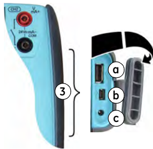
Figure 1-3: The USB and power sockets
