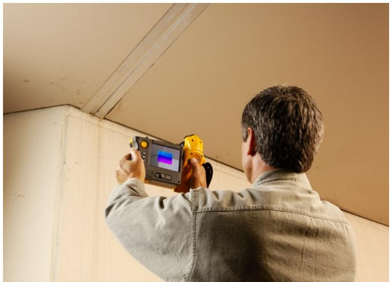
minutes after the first spray test, it took almost an hour for the cooler evaporative temperatures to reach the surface of the interior wall.
