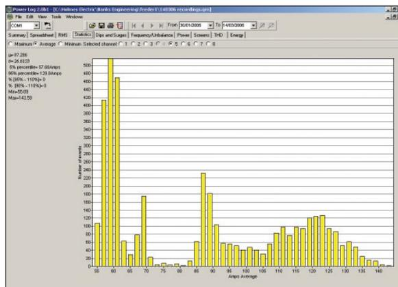
Figure 5. Power Log statistics view showing average current.
