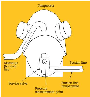
**Figure 3.** Suction line superheat using the temperature-pressure method. Measure the pressure at the suction line service valve. Find the evaporator boiling temperature from a temperature-pressure chart using suction line pressure. Subtract this temperature from the suction line temperature measured by the Fluke digital thermometer. The difference is superheat.
