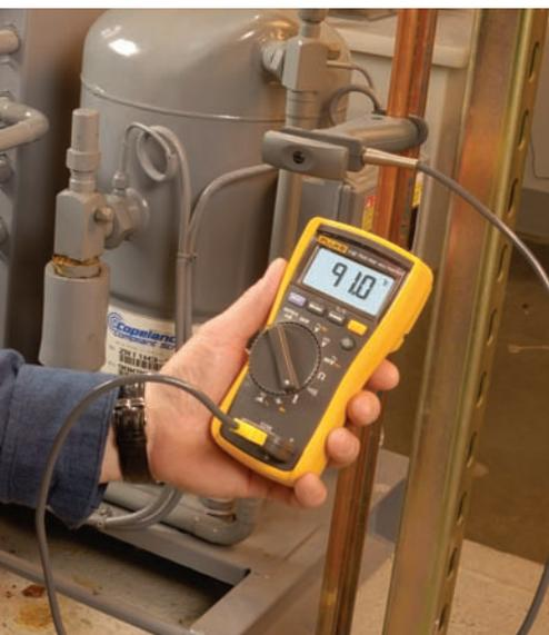
Measuring liquid line temperature with a DMM and a pipe clamp.
