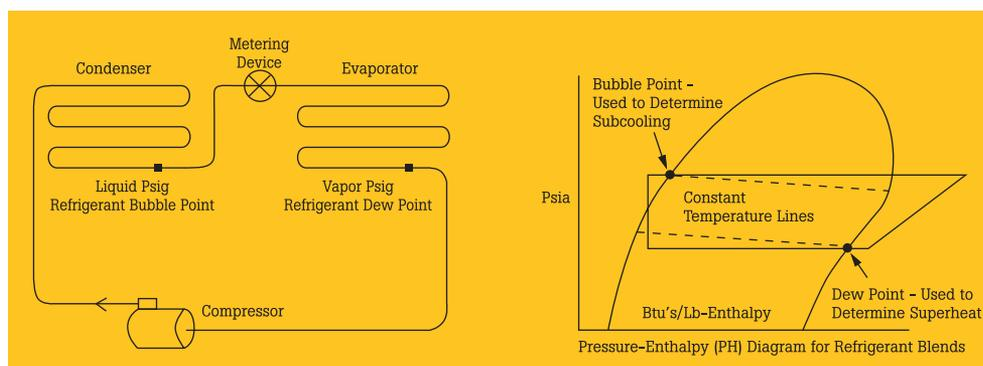
**Figure 2.** Superheat temperature measurement points.
