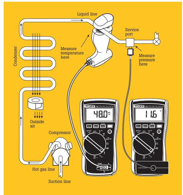
**Figure 5.** Subcooling. After verifying normal airflow, place the pipe clamp or Velcro probe on the liquid line. Note the temperature. Then attach the pressure/vacuum module to a port on the liquid line and measure the liquid line pressure. Determine the condensing temperature by using the temperature-pressure chart for the refrigerant type used. The difference in temperature is the subcooling value.
