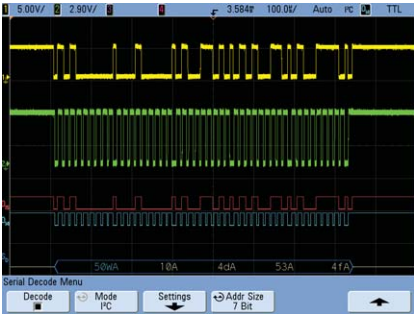
View on-screen serial decode of an I 2 C packet.
