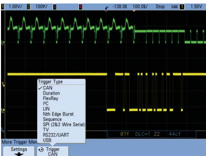
Trigger on and decode CAN serial packets.
