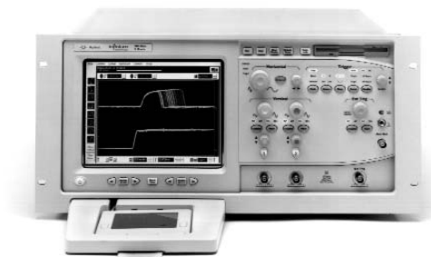
Figure 12.2. Infiniium scope ready to fit into EIA standard 19-inch cabinets.
