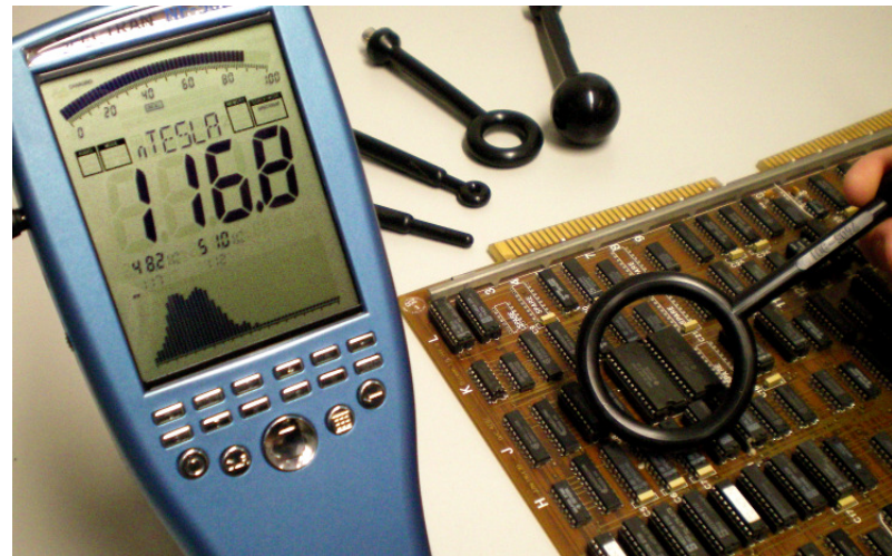
Magnetic field measurement on a group of components using the 60mm H-field probe
