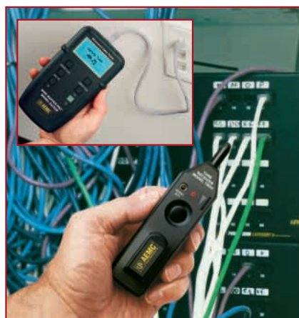
Model TR02 used to find cables in a panel.
