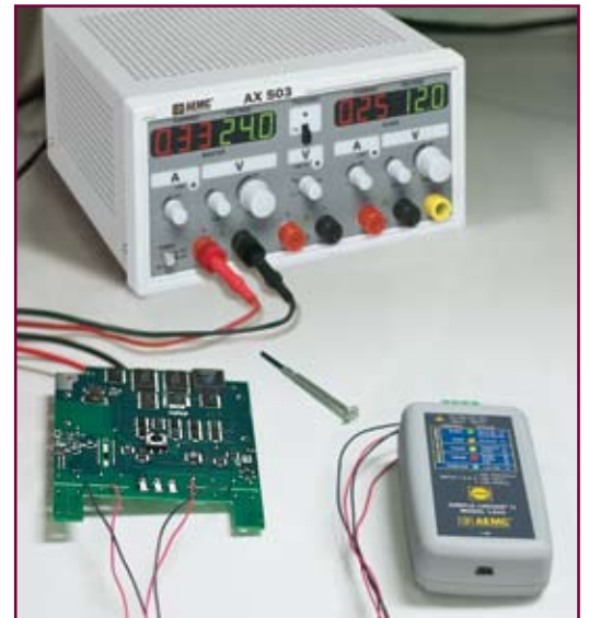
L432 recording two DC voltage supplies.
