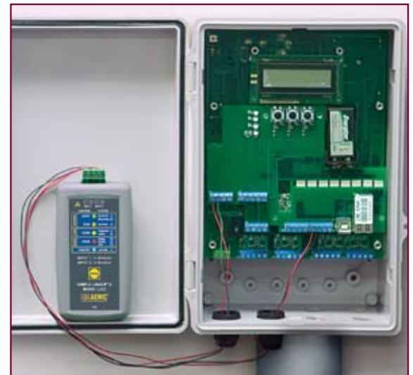
L322 recording loop current in a flow control panel.
