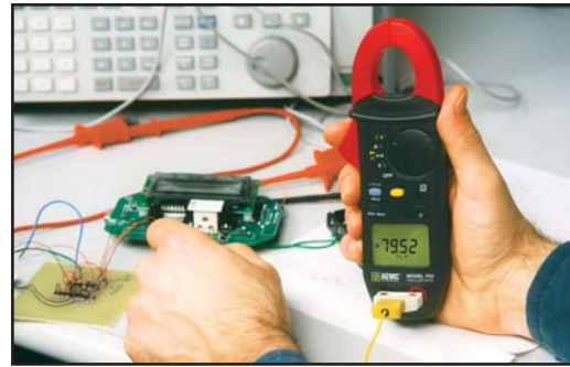
Model F03 measuring temperature on electronic circuit board using a K thermocouple.
