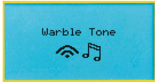
Built-in tone generator for cable tracing.
