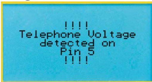
Automatic detection of live telephone voltage.
