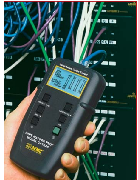
Model CA7028 at patch panel verifying cable runs.
