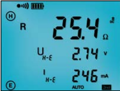
The 4-Point Bond test displaying lead connections, bond resistance test results, test voltage and current.
