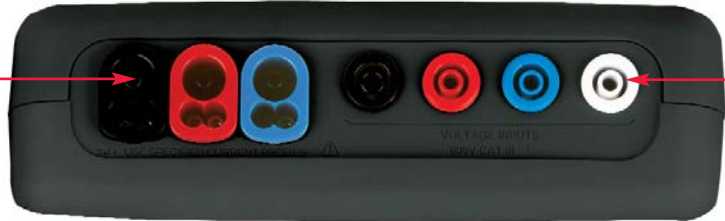
The color-coded input connectors provide dedicated current probe inputs and voltage inputs.
